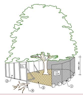
1. CHAIN WIRE MESH PANELS WITH SHADE CLOTH (IF REQUIRED) ATTACHED, HELD IN PLACE WITH CONCRETE FEET
