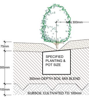
**TYPICAL GARDEN PREPARATION DETAIL** SCALE 1:10 (ONLY APPLICABLE FOR PLANTING AREA OUTSIDE TREE PROTECTION ZONE OF TREES TO BE RETAINED. NO CHANGES ARE TO OCCUR TO EXISTING LEVELS, INCLUDING RIPPING/CULTIVATING OF THE SOIL WITHIN THE TPZ OF TREES TO BE RETAINED ON SITE)
